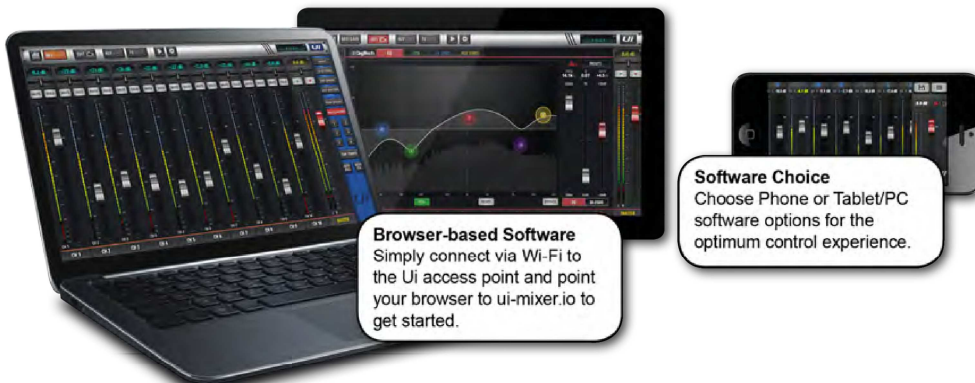
WiFi Antenna / LED WiFi access point to built-in web server enables browser-based software control.
